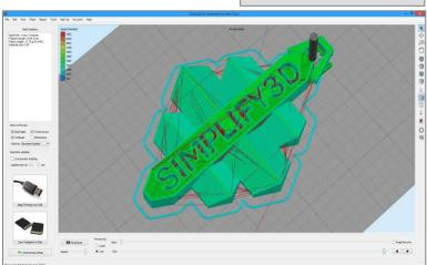
• Start and End Slider Bars: Allow you to move through the Preview manually. (Hint: leave the Start slider positioned left and drag the End slider right to view the build sequence.)
